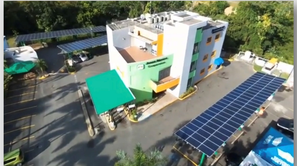
Aerial view of JOC building, presenting the Photovoltaic System that produce 96.5 KWh of clean energy. Since inception in 2015, has produced 600 MWh, equals to avoid to produce 359 Tons of Carbon Bioxide. Its savings totaled up to 86% in cost of energy.
